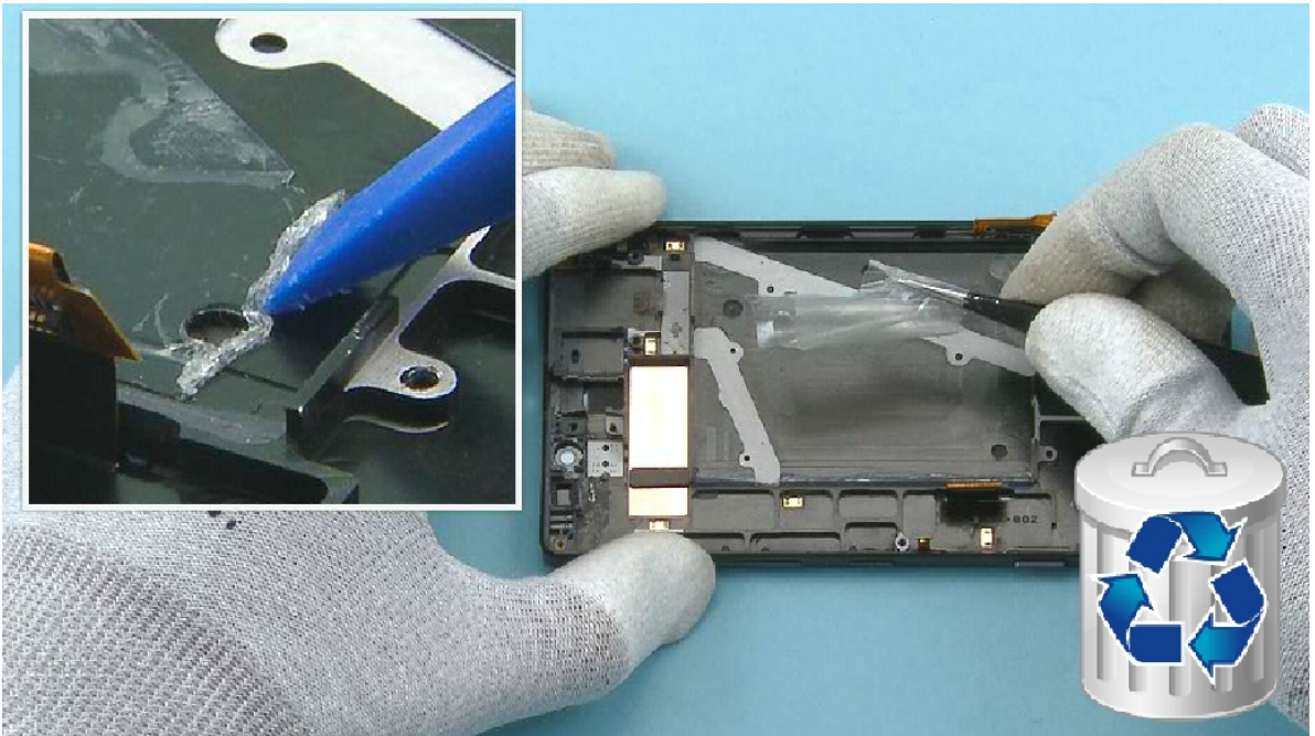
43) Peel off and discard the BATTERY ADHESIVE using SS-93 and tweezers
