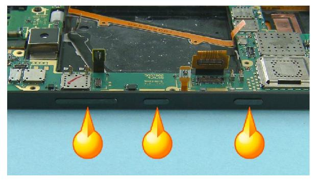
29) After assembling the ENGINE BOARD check the tactility of the side keys.
