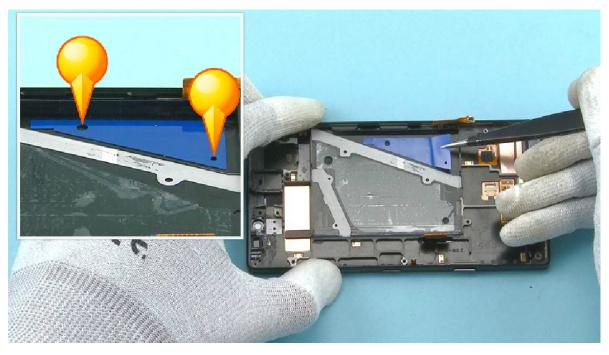
10) Place the SMALL BATTERY ADHESIVE as shown on the UI ASSEMBLY. Use the shown holes to get the right alignment.
