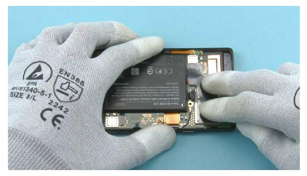
35) Press all around the HEAT SPREADER to activate the adhesive.
