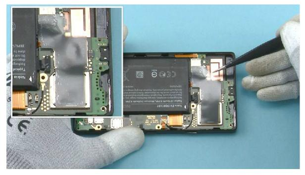
34) Place the HEAT SPREADER on the ENGINE BOARD as shown. Use the edges of the shielding lids to get the right alignment.
