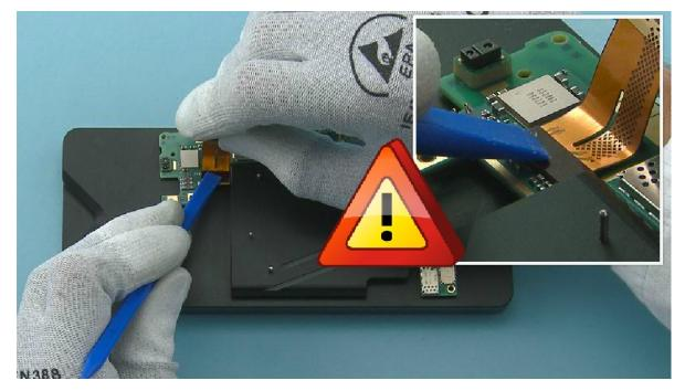
25) Connect the CAMERA to the ENGINE BOARD with the SS-93. Be careful not to damage the connector or any components nearby.
