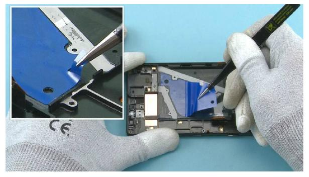
9) ... and peel off the protective film.
