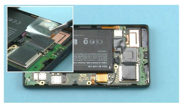
36) Remove the protective film and gently press all around the HEAT SPREADER again to make sure its properly attached.
