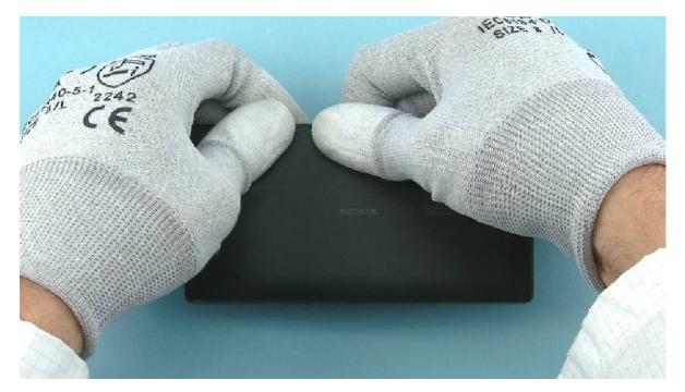
41) Then press together all the other sides of the device to get the BACK COVER completely attached.
