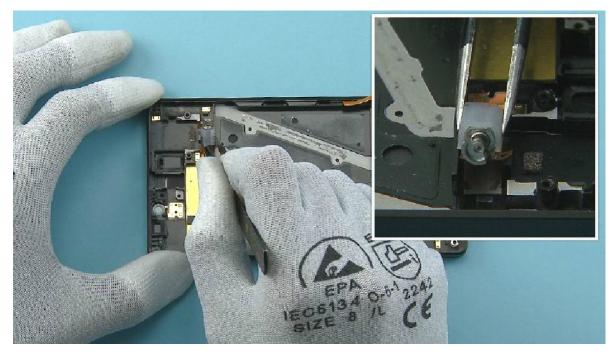
14) Place the VIBRA ASSEMBLY to its slot on the UI ASSEMBLY. First align the flex to its place, then lower down the VIBRA.
