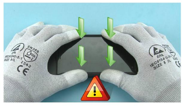
20) Then place the UI ASSEMBLY on the jig and press it gently but properly to get the flexes attached. Be careful not to damage the DISPLAY.
