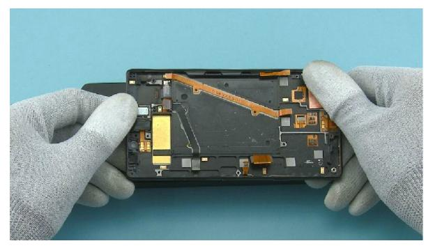
21) Remove the UI ASSEMBLY from the jig and check that the flexes are properly attached.
