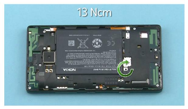
38) Fasten the TORX+ SIZE 4 screw to the top of the BATTERY CONNECTOR STRAP to the torque of 13 Ncm.
