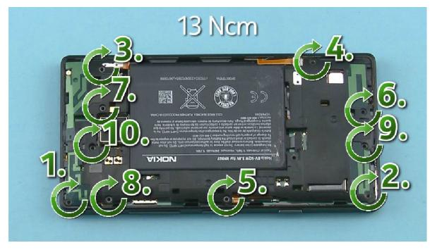
37) Fasten the ten TORX+ SIZE 4 screws in the order shown to the torque of 13 Ncm.
