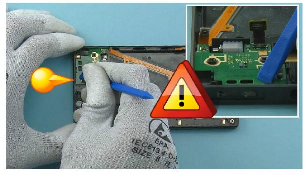
23) Then lower down the DAUGHTER ENGINE BOARD and press down to attach the shown clip. Be careful not to damage the DAUGHTER ENGINE BOARD or any of its componets.
