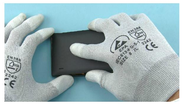
39) Assemble the BACK COVER to the UI ASSEMBLY bottom end first.
